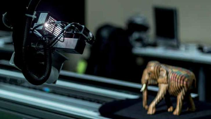
When combined with **CultArc3D**, **CultArm3D** is used to capture remaining holes, occlusions or geometrically complex surface areas in more detail.
